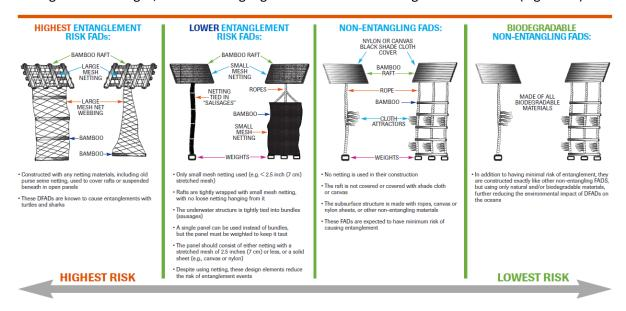
Figure 17: ISSF ranking of FAD designs from highest to lowest risk of entanglement (from ISSF, 2015b)
