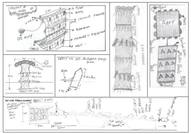
Figure 14: Observer drawings of commonly used FAD designs in the WCPO.
